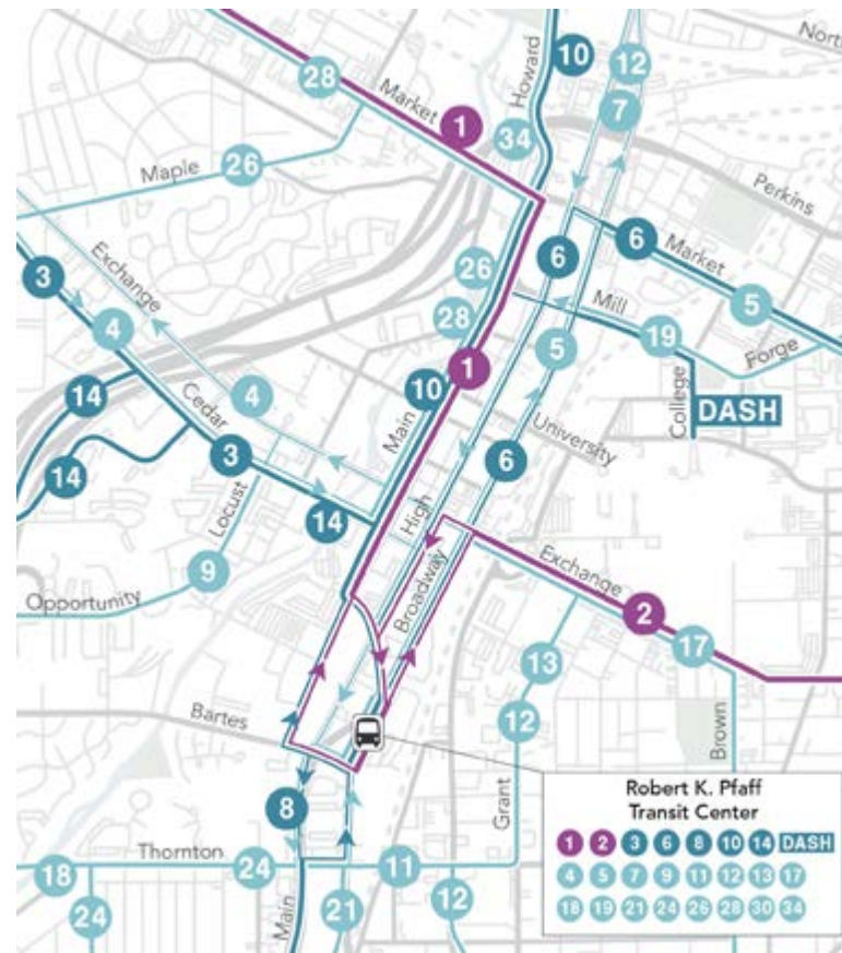
Figure 27: Because there are only a few available paths for transit, duplication in Downtown Akron is an outcome of the network's radial structure and focus on RKP Transit Center.
